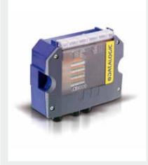
The CBX800 industrial connectivity device serves as a gateway, connecting devices equipped with a standard RS232 communication interface to the most common fieldbus systems, through a complete range of option module options, in addition to an ID-NET™ high speed communication network.
