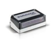
The DS100 embedded bar code reader is a cost-effective laser scanner characterized by ultra-compact dimensions, motor on/off software commands, wide reading width at a short reading distance, lightweight design (<100 g), built-in RISC decoder, scanning speed of 500scans/sec, dual high speed serial interface, and IP65 rugged industrial housing.
